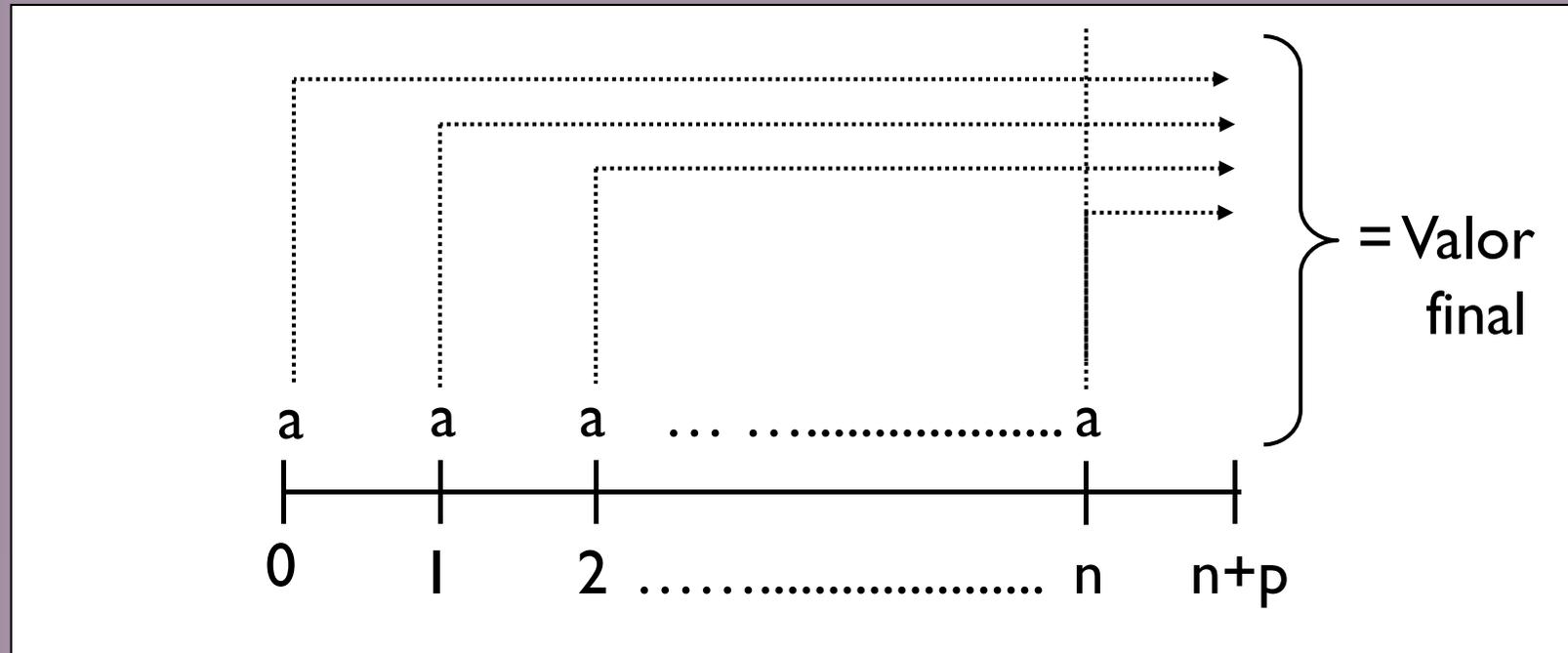
$$\text{Valor final} = p / a \cdot \ddot{S}_{\overline{n}|i} = a \cdot \ddot{S}_{\overline{n}|i} \cdot (1+i)^p$$
