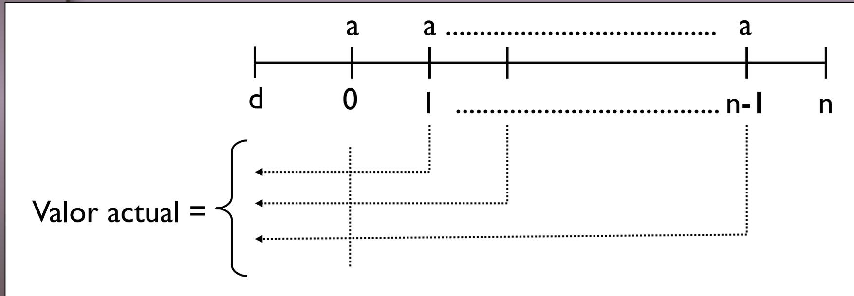
$$\text{Valor actual} = d / a \cdot \ddot{a}_{\overline{n}|i} = a \cdot \ddot{a}_{\overline{n}|i} \cdot (1+i)^{-d}$$
